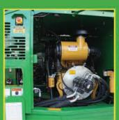
Accessible engine bay Provides excellent accessibility to the traverse mounted 225hp Tier III CAT diesel engine and hydraulics.
